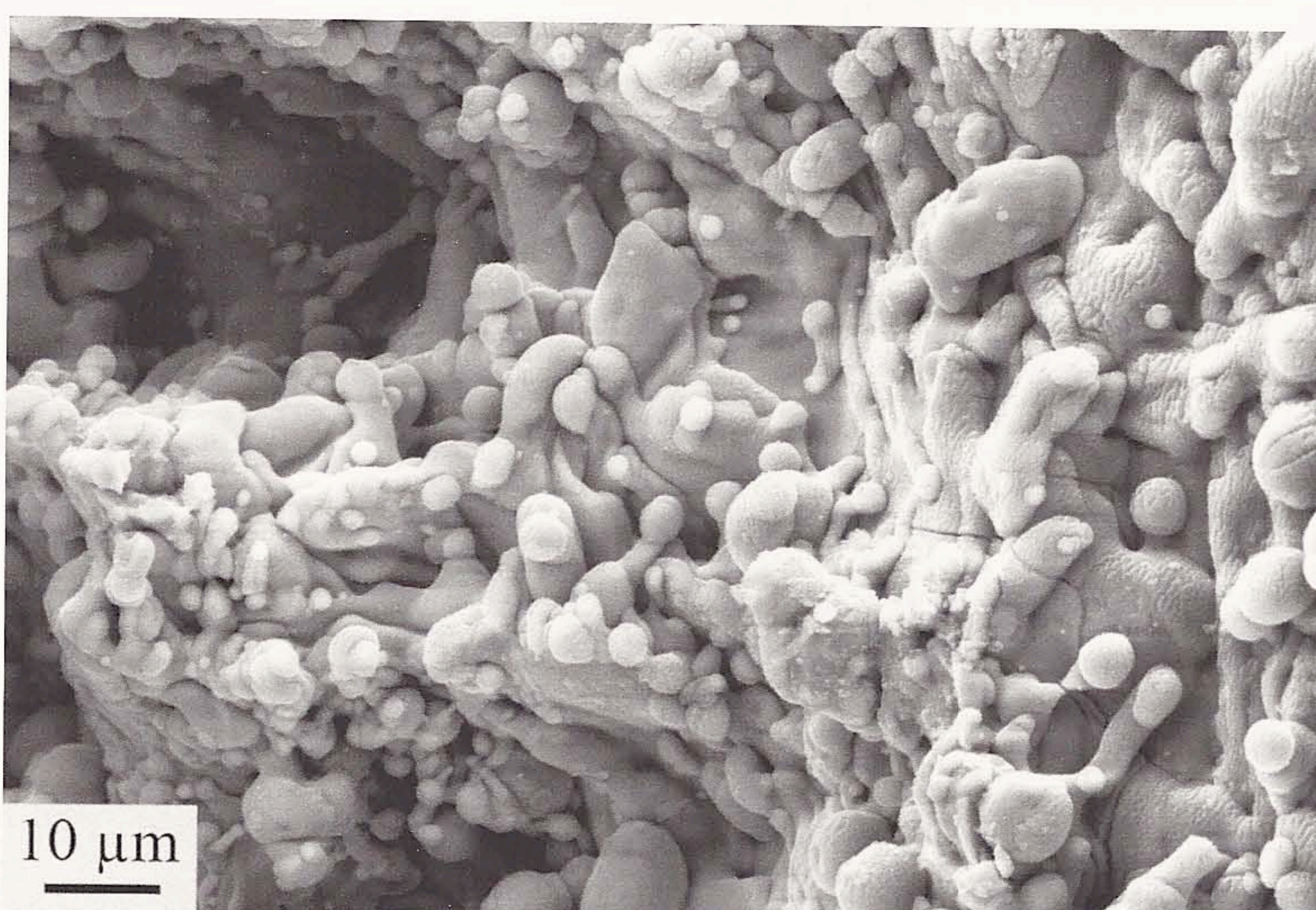
Fig 2 Scanning electron microscope micrograph at 1000X magnification showing the resolidified material from the laser processing.
